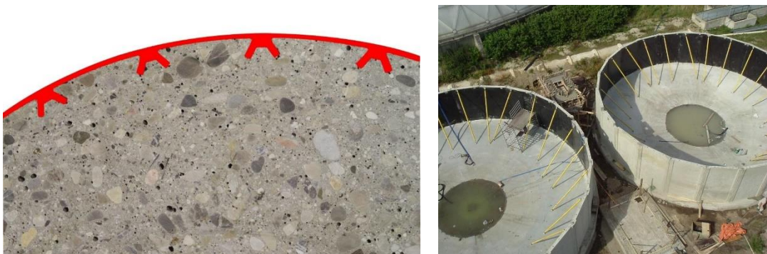
(l) Agru Sure Grip doorsnede , (r) Agru Sure Grip in de waterzuivering
